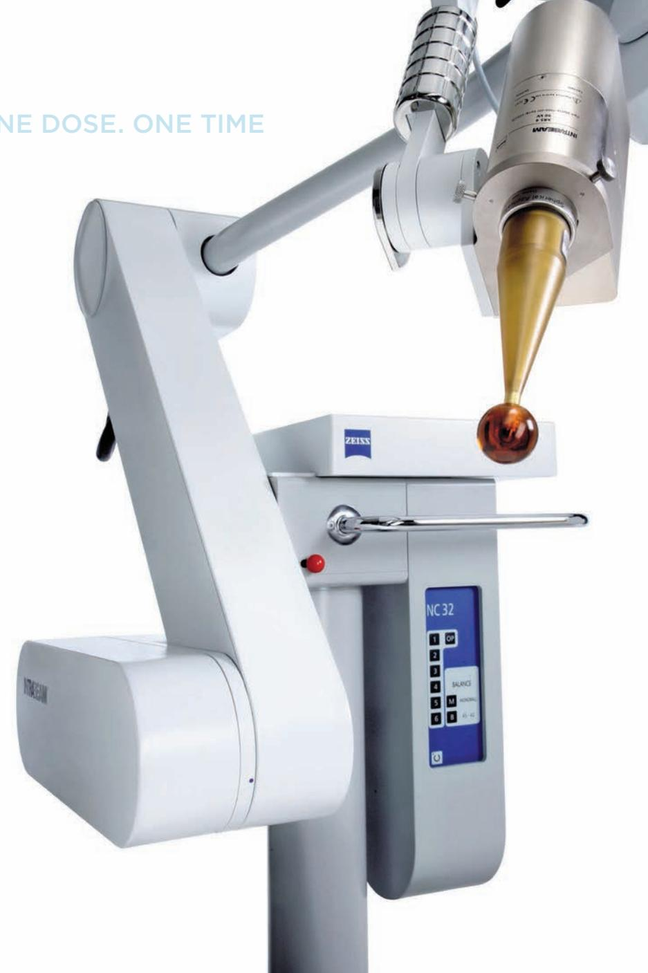
**Figure 2.** INTRABEAM system used for delivery of intraoperative radiotherapy.
