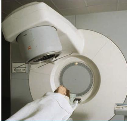
**Figure 1.** Linear accelerator used to deliver conventional external beam radiation.
